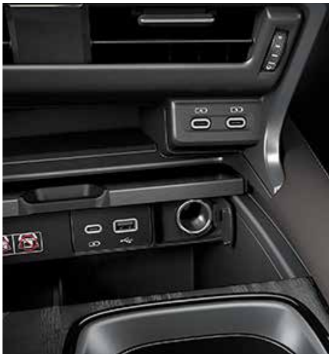
Center console: 3 USB Type C charging and USB Type A multimedia communication ports, DC12V
